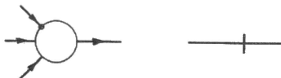
GATE, WITH INHIBITOR INVERTER (OR 'NEGATE')
