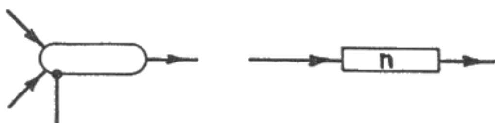
TRIGGER, (WITH 2 INPUTS) DELAY OF n UNITS
