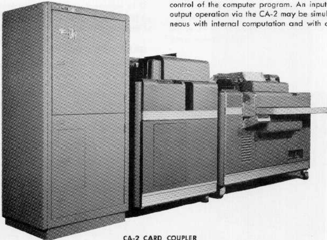
CA-2 CARD COUPLER WITH TYPICAL PUNCHED CARD EQUIPMENT
